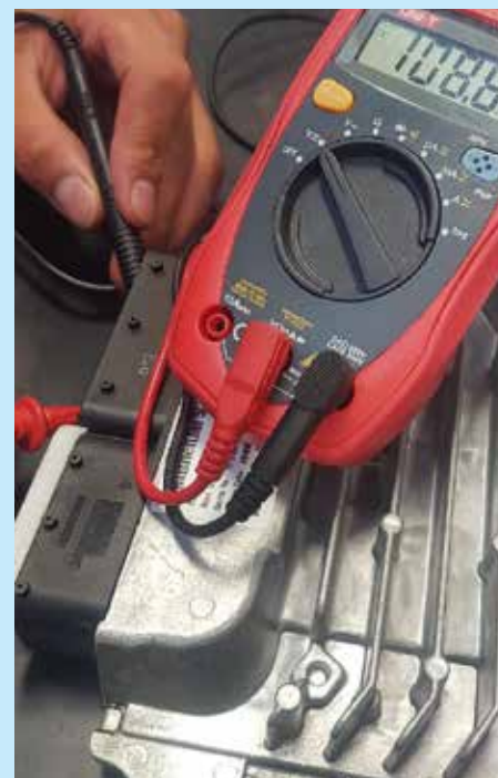
Measuring the resistance of a circuit in an electronic control unit.
