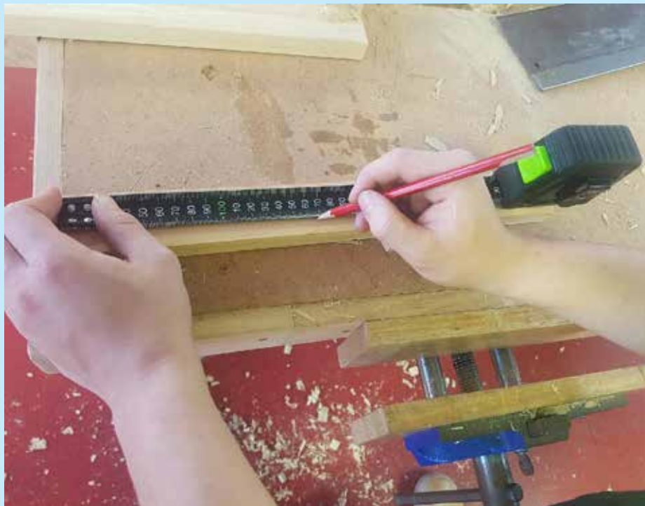
Using a tape measure to find the length of wood for a toolbox project.
